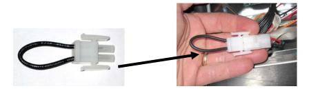
8. Plug the new supplied harness into the male end of the two-pin plug drain switch, unplugged in step 6, with the brown and black wires. Refer to wiring diagram on the following page.
