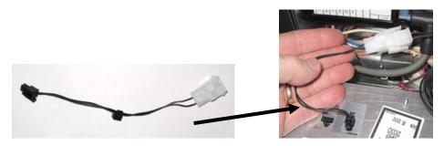
9. Install the new controller into the slots. Plug the 20-pin plug and the new 4-pin harness, attached in step 8, into J4 on the controller as shown in the photo below. Attach the ground wire to the corner spade shown below.
